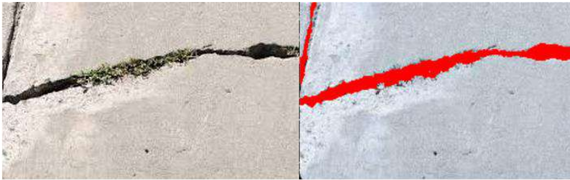
Figure 12 Original digital data: and segmented data with Random Walker and Graph cut
