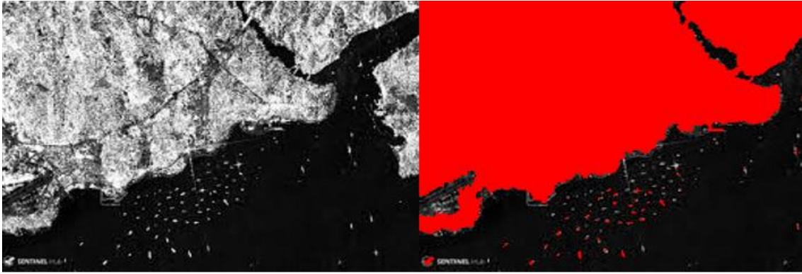
Figure 10 Original Radar data: and segmented data with Random Walker and Graph cut
