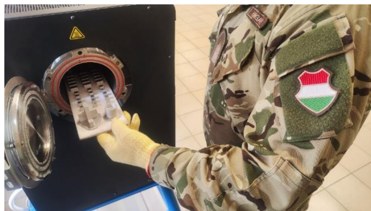
Figure 2. Removal of printed metal parts made by ADAM technology from the sintering furnace
