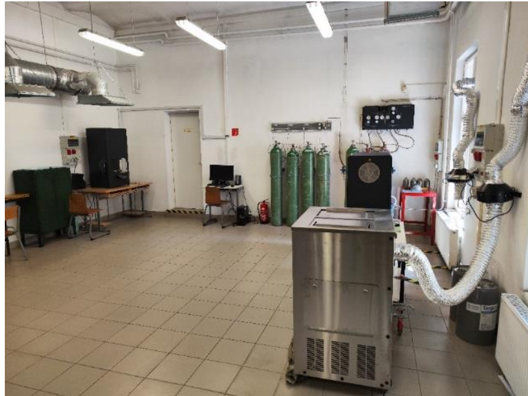
Figure 1. 3D metal printing laboratory with ADAM technology: the printer in the left corner, the washer in the foreground, sintering furnace, and the gas supply system in the background
