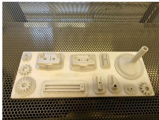
Figure 5. Various machine components (gear, coupling, valve, etc.) on the ceramic tray of the sintering furnace
