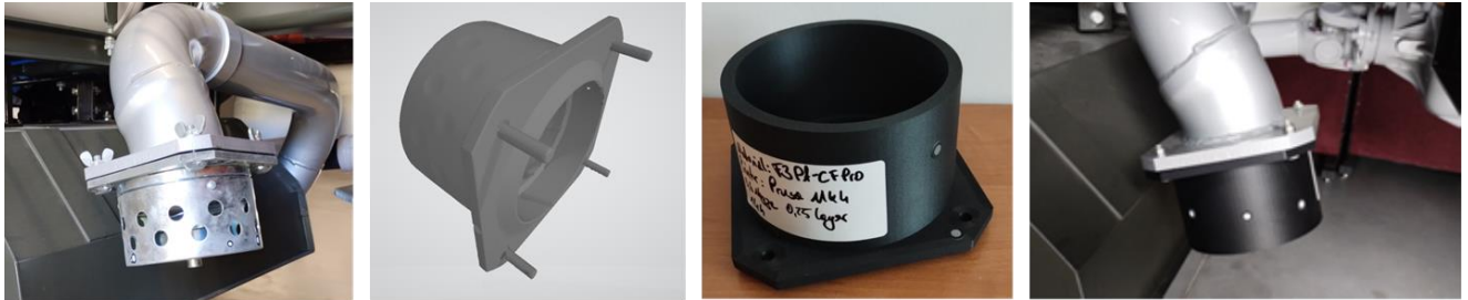
Figure 3. From original part, through scan, print to replacement part source: from the archives of K. Kowalski
