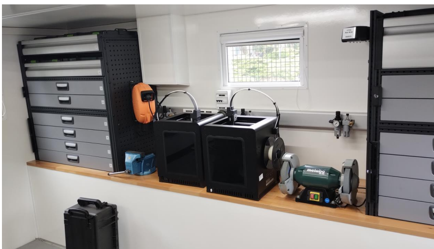
Figure 4. A mobile universal containerized service and repair workshop equipped with a scanner and 3D printers
