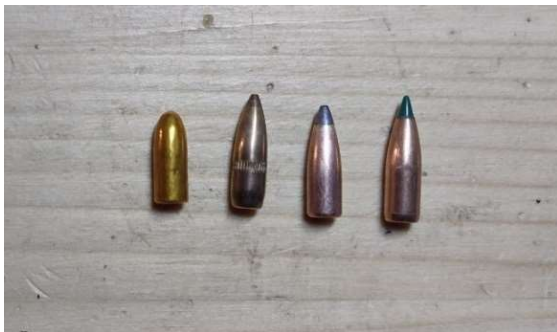
Fig. 2 Types of bullets which were use in experiment. From left to right: RN type, FMJ type, SP type and Blitzking design Source: authors.
