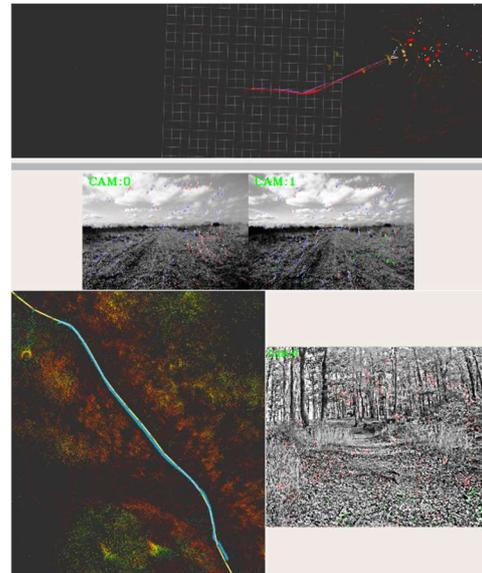
**Fig. 14** Visual odometry using OpenVINS [35] - top: on Rellis-3D [2] dataset (red - ground-truth trajectory, purple - OpenVINS odometry); bottom: on our dataset (yellow - ground-truth trajectory, cyan - OpenVINS odometry)
