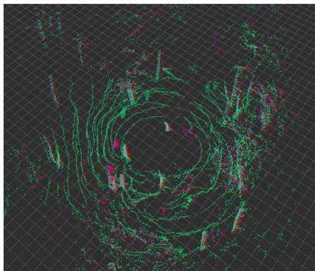
**Fig. 5** Refining of the resulting transformation using GICP - current point-cloud transformed according to ScanContext recognition (red), point-cloud of the recognized site (green), point-cloud after transformation refinement (purple)
