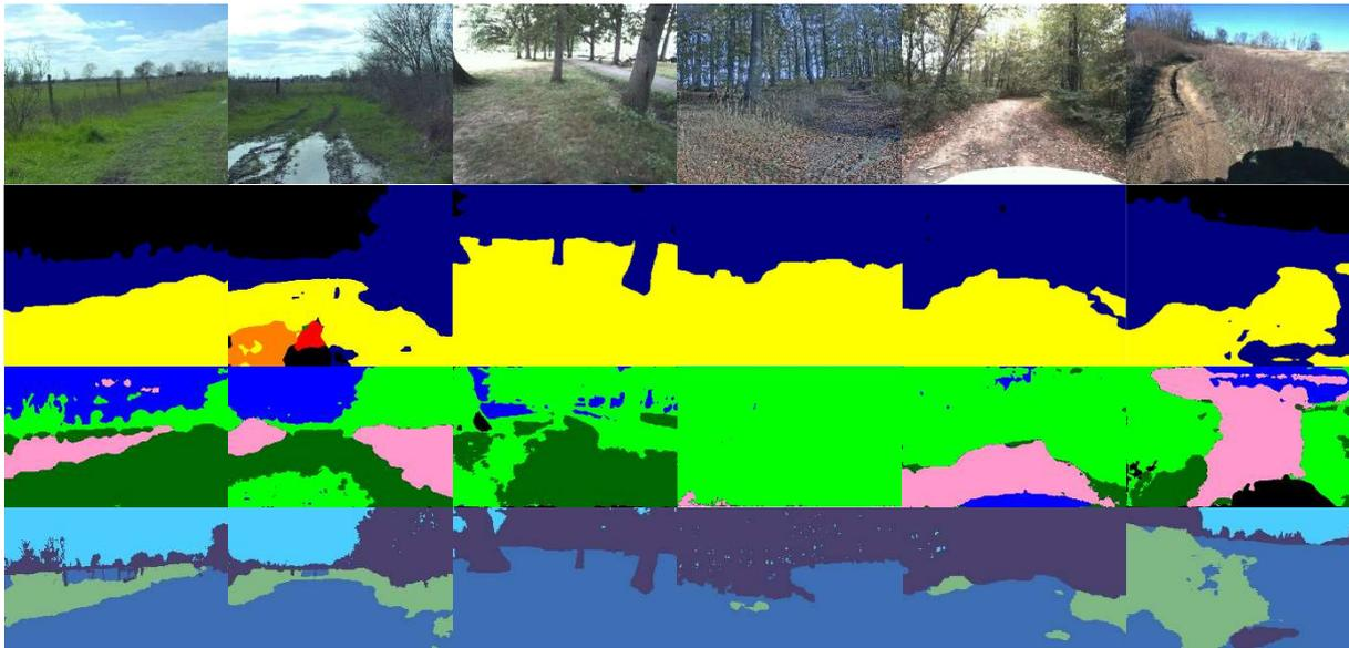
**Fig. 16** Traversability segmentation of an image. First row: segmented images (from RELLIS-3D [2], Yamaha-seg [3], and our dataset). Second row: segmentation using GANav [39] model trained on RUGD [1] dataset. Third row: Unet [40] model trained within Traversability estimation [12, 13] project on RELLIS-3D [2] dataset. Fourth row: BiSeNet [41] model trained within OFFSEG [42] project on RUGD [1] dataset
