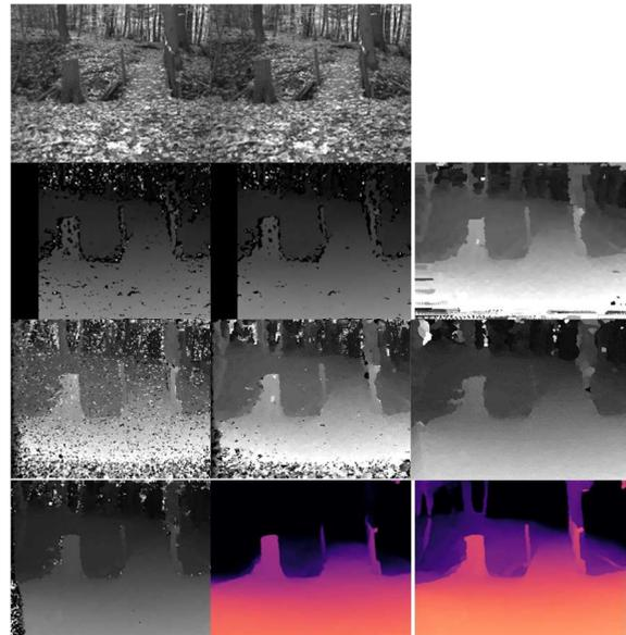
**Fig. 10** Depth estimation. First row (left-to-right): left camera image, right camera image [15]; Second row: depth estimated by BM [16], SGBM [17], ASW [18] algorithms; Third row: AD-Census V1 [19], SAD [20], ZNCC [21]; Fourth row: SGM [22], ACVNet [23] trained on SceneFlow [24] dataset, HITNet [25] trained on Middlebury [26, 27, 28, 29, 30] dataset
