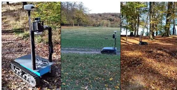
**Fig. 2** RTV Crawler mobile platform with sensoric setup in different environments during recording of our dataset
