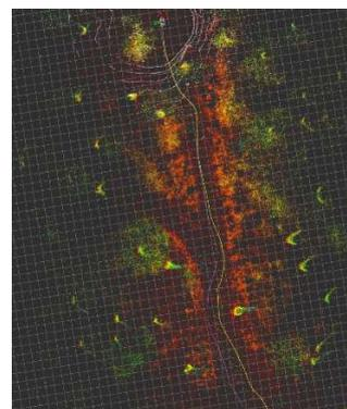
**Fig. 3** NDT LiDAR odometry (yellow) compared to ground-truth UGV trajectory (purple) – locally it is highly accurate and consistent, although (like in the case of any odometry) its deviation increases gradually
