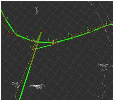
**Fig. 4** A successful loop-closure marked by a short thick orange line between two nodes of a pose graph
