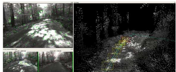
**Fig. 15** Detection of a previously visited site and loop closure using RTAB-Map
