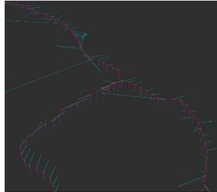
**Fig. 6** Pose graph with odometry (red), loop-closure (orange), GPS (cyan), and IMU (purple) measurements
