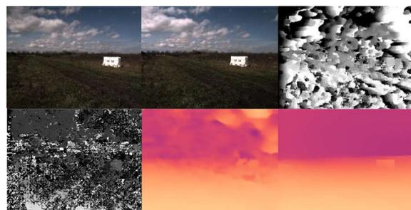
**Fig. 11** Depth estimation from an uncalibrated stereo-pair of images. First row (left-to-right): left camera image, right camera image [2], depth estimated by ASW algorithm; Second row: SGM, ACVNet trained on KITTI [31, 32] dataset, HITNet trained on Middlebury dataset
