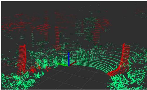
**Fig. 8** Traversability estimation of a point-cloud using DeepLabv3 ResNet101/TraversabilityClouds
