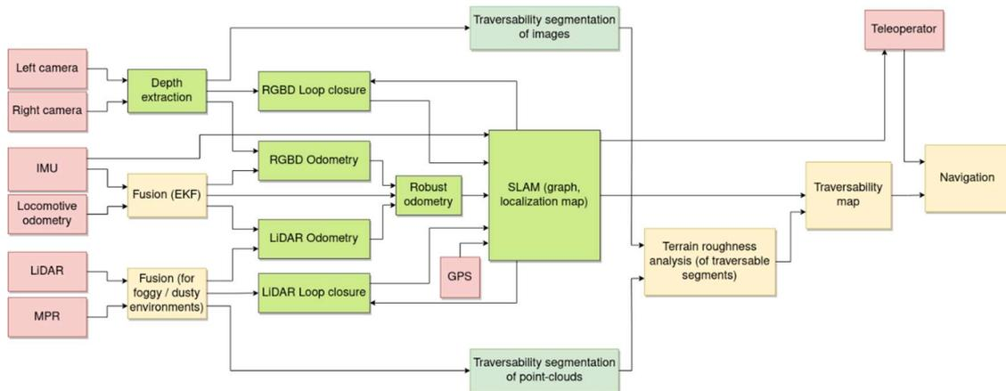
**Fig. 17** Outline of the perception system and its application onto UGV navigation; red - inputs, green - perception system components analyzed in this work (pale green - second phase), yellow - other components of navigation system
