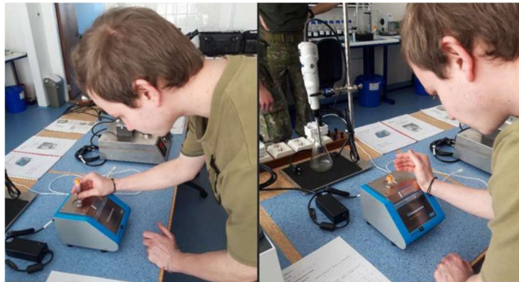
Fig. 12 Method of loading the sample into the FerroCheck 2000 device Source: authors.
