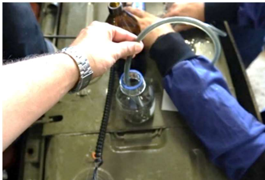
Fig. 8 Method of oil sampling Source: authors.
