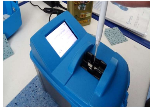
Fig. 16 Application of oil sample Source: authors.
