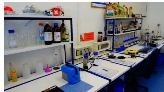
Fig. 2 Tribodiagnostic Laboratory - SpectroVisc Q3050-blue, Spectro Q1000 Fluidscan-yellow Source: authors.
