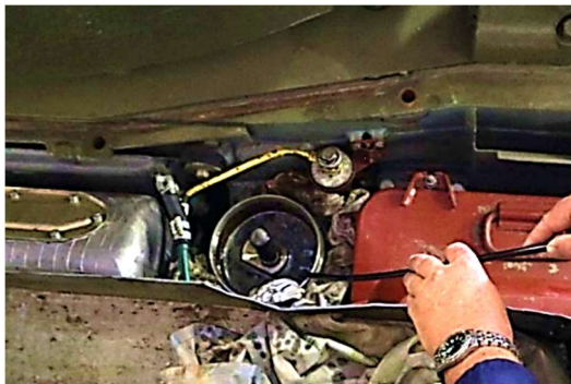
Fig. 7 Oil sampling from MAF cleaner Source: authors.
