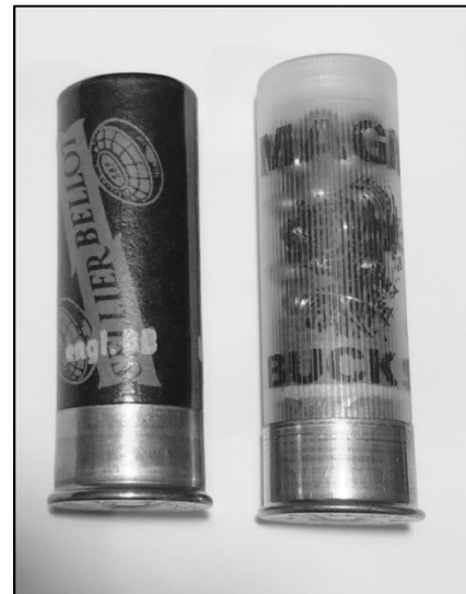
Fig. 1 #1 Birdshot (left) and #4 Buckshot (right) shells
