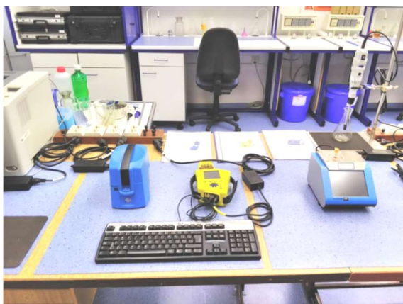
Fig. 8 Laboratory of Tribodiagnosics-SpectroVisc 3050-blue, Spectro Q 1000 Fluidscan-yellow, Ferro Check 2000-blue with screen Source: authors.
