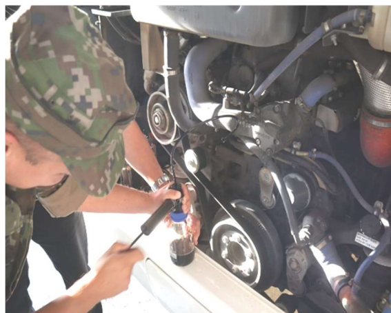
Fig. 2 MO sampling from the vehicle engine Source: authors.
