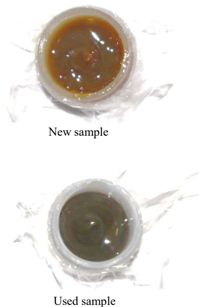
Fig. 13 PM Total Ceran, NLGI 0 Comparison of Reference and used sample Source: authors.
