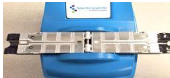
Fig. 11 SpectroVisc TriboVisc measuring cell 3050 Source: authors.
