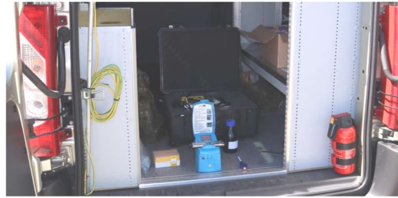
Fig. 10 In-vehicle COPMBO measurement kit Source: authors.
