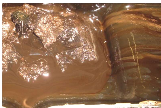
Fig. 6 Demonstration of MO degradation by fuel and ethylene glycols Source: authors.
