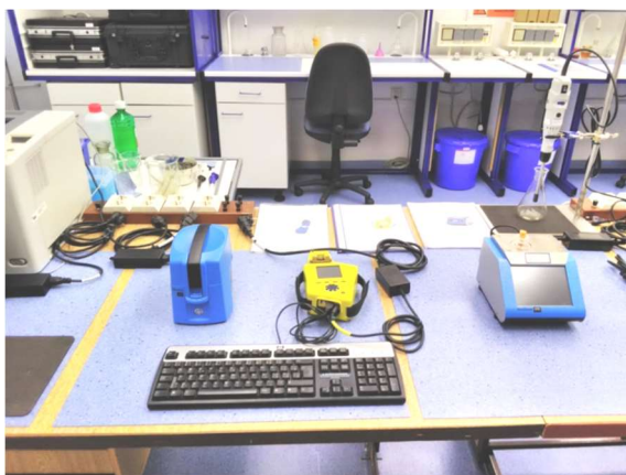
Fig. 8 Laboratory of Tribodiagnostics-SpectroVisc 3050-blue, Spectro Q 1000 Fluidscan-yellow, Ferro Check 2000-blue with screen Source: authors.
