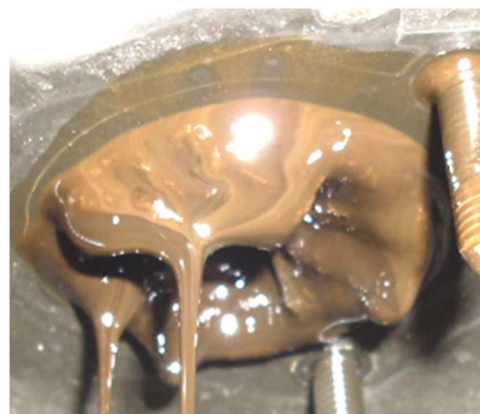
Fig. 7 Demonstration of MO degradation at contamination with ethylene glycols (Ethylene Glycol- C_2H_6O_2 , or Propylene Glycol- C_3H_8O_2 ), also at sulfation Source: authors.
