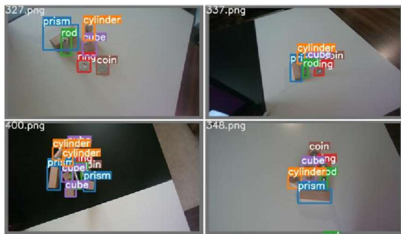
Fig. 9 Output of the trained neural network on a series of test images from the dataset Source: author.
