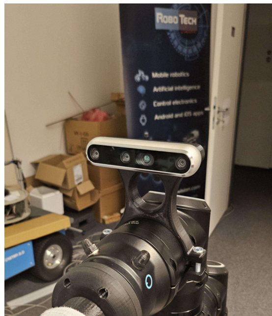
Fig. 2 Placement of the Intel RealSense D455 camera on the Spinbotics Robotic Arm Source: author.
