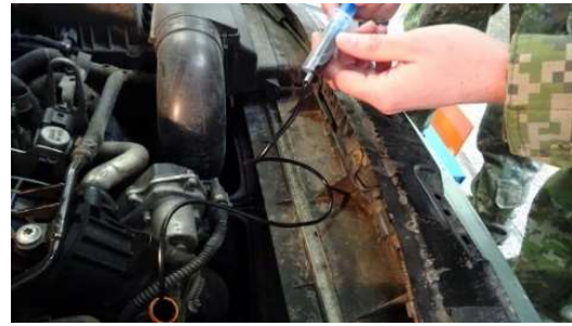
Fig. 4 Sampling MO – Castrol Edge 5W -30 Source: author.
