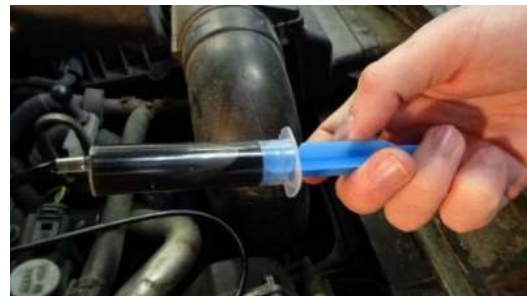
Fig. 5 Sampling with syringe Source: author.
