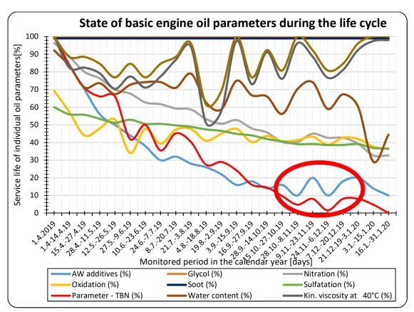
Fig. 5 Illustrative example service life of engine oil in an internal combustion engine and the most fragile parameters (parameter TBN, AW additives) [1] Source: authors.
