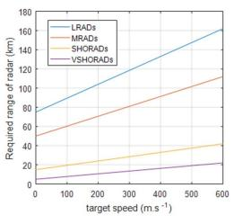
Fig. 2 Required radar ranges vs. target speed. Source: authors.
