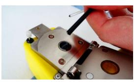
Fig. 9 Inserting the sample on the sample slide 2 Source: authors.
