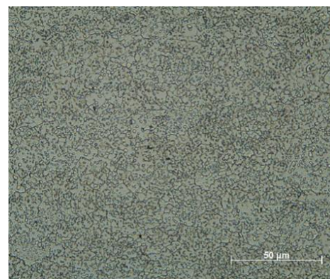
Fig. 1 Microstructure of 100MnCrW4 steel Source: author.
