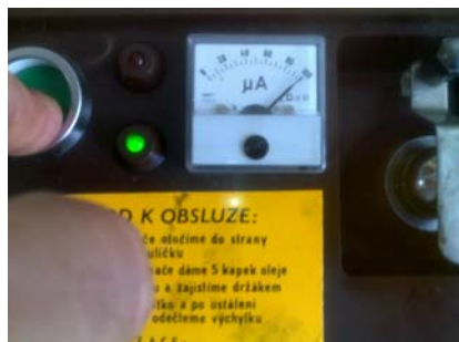
Meranie prietoku \mu\text{A} cez MO Castrol EDGE Profesional LongLife III, 5W-30
