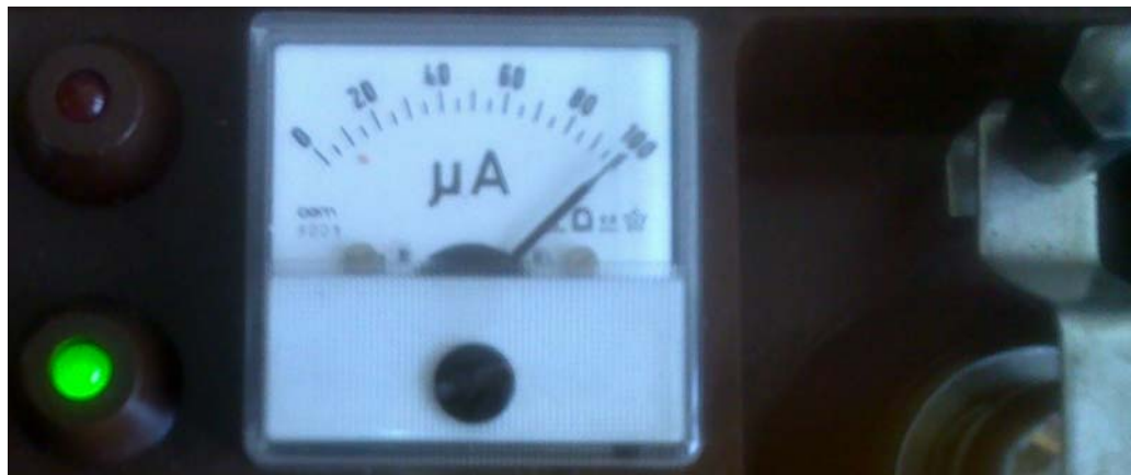
Meranie prietoku \mu\text{A} cez MO Castrol EDGE Profesional LongLife III, 5W-30
